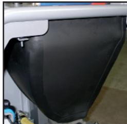
Insulated pellet hopper with 23 kg (50.71 lbs) capacity
